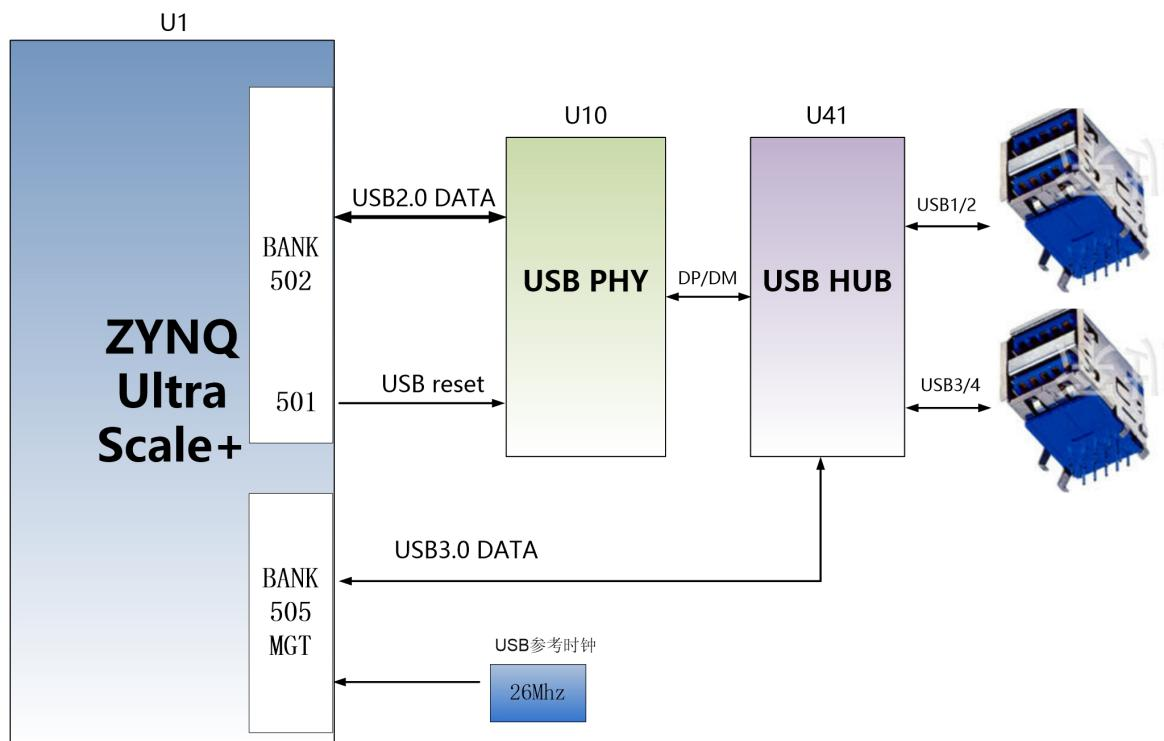
Figure 8-1: USB 3.0 Schematic
