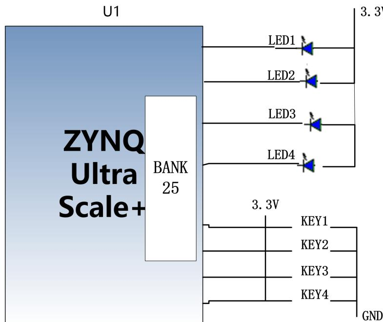
Figure 17-1: LED Schematic
