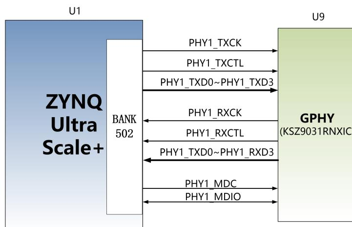
Figure 9-1: ZYNQ PS System and GPHY Schematic
