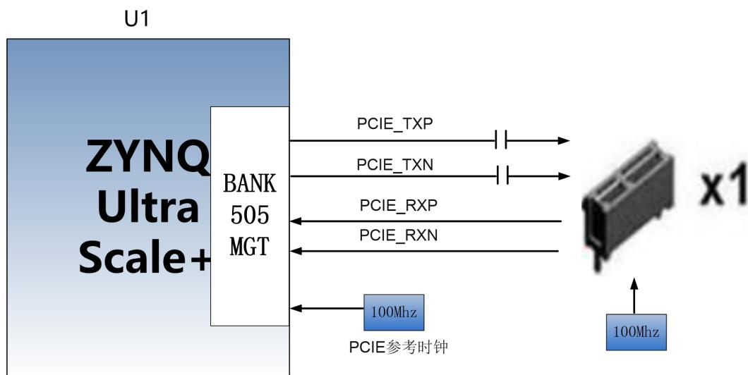
Figure 12-1: PCIE Schematic
