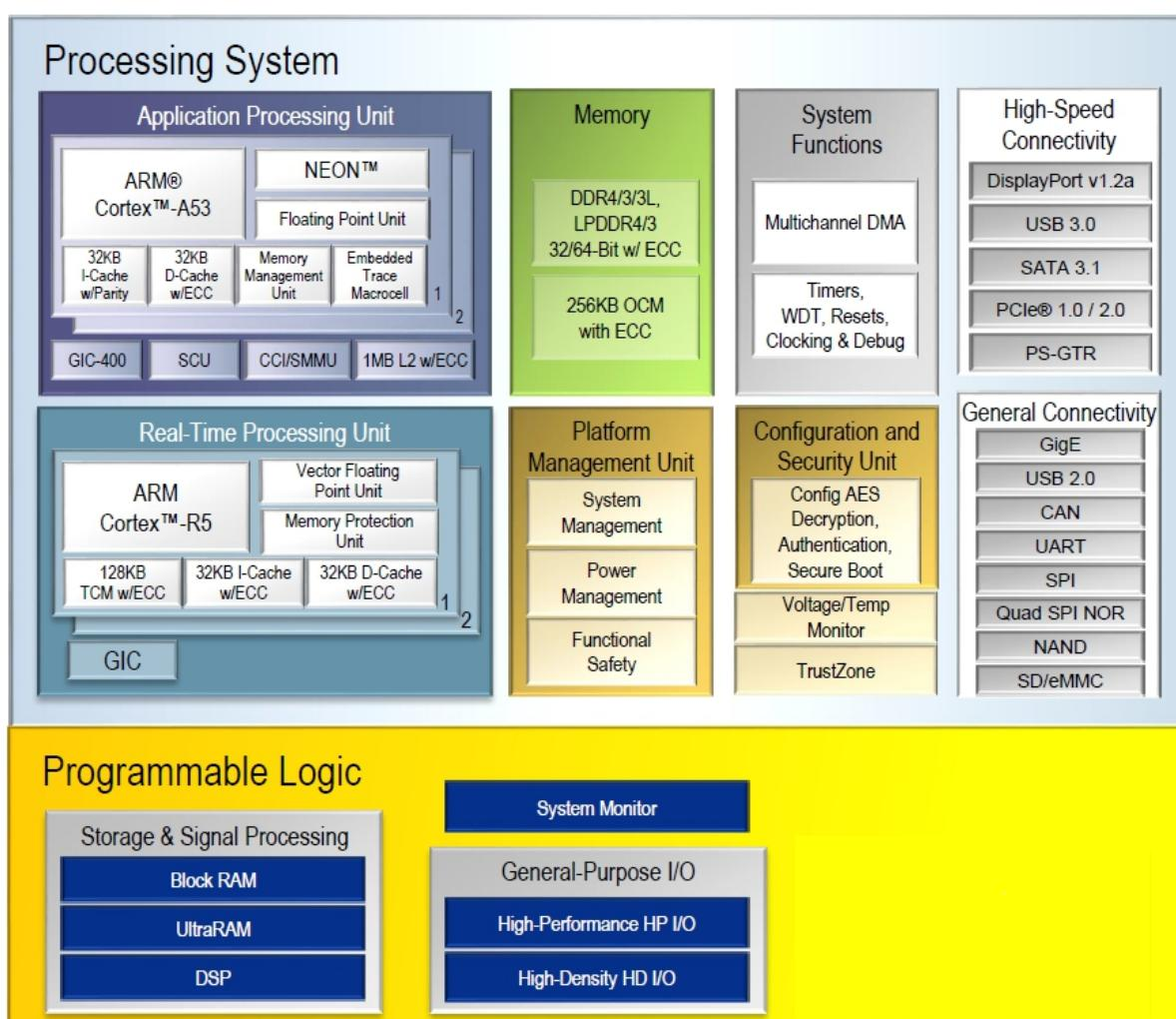
Figure 2-1: Overall Block Diagram of ZU2CG Chip
