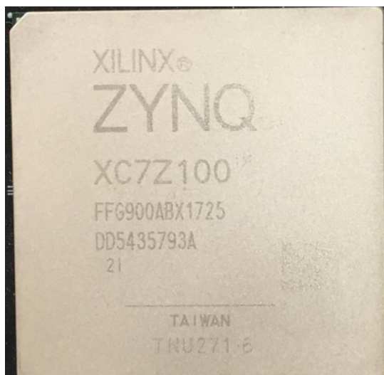
Figure 2-2-3: The XC7Z100 chip used on the Core Board
