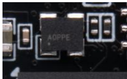
Figure 2-5-2: 33.333333Mhz active crystal on the core board
