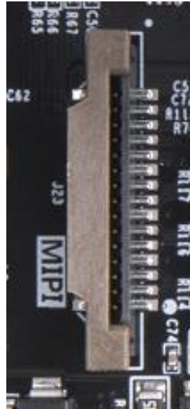
Figure 3-9-2: MIPI camera interface on the carrier board
