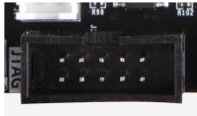
Figure 3-14-2: JTAG Interface on the Carrier Board
