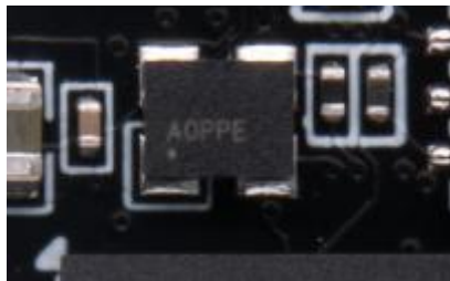
Figure 2-5-2: 33.333333Mhz active crystal on the core board
