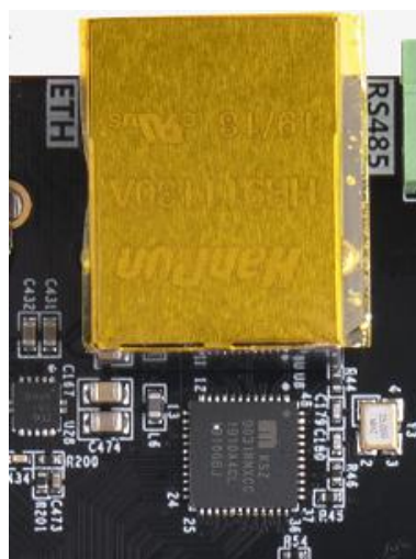
Figure 3-4-2: Ethernet GPHY chip and interface on the carrier board
