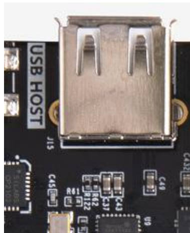
Figure 3-5-2: USB2.0 on the carrier board
