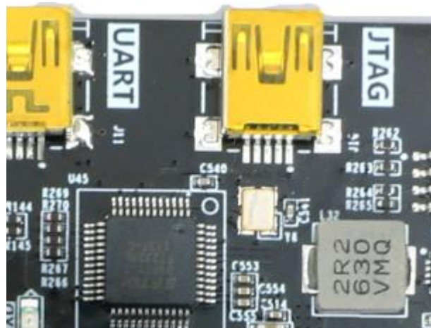
Figure 17-2: JTAG Interface on the AX7350 FPGA Board
