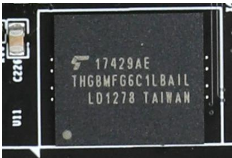
Figure 5-2: eMMC Flash on the AX7350 FPGA Board
