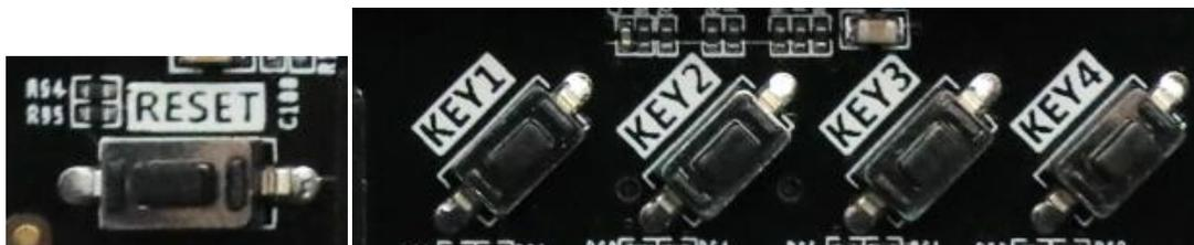
Figure 20-2: Reset Key and User Keys on the FPGA Board
