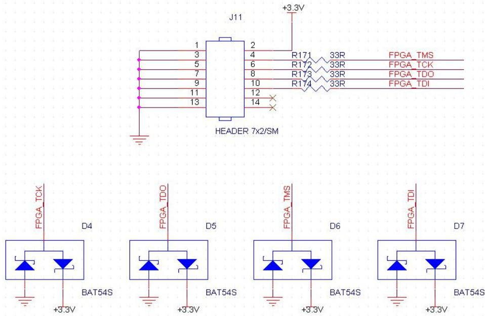
Figure 19-1: JTAG Interface Schematic
