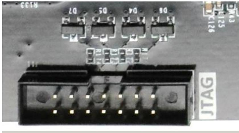
Figure 19-2: JTAG Interface on the FPGA board
