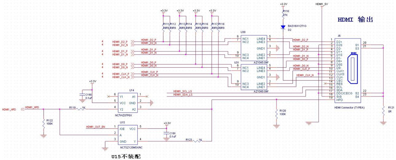
Figure 9-1: HDMI Output Interface Schematic
