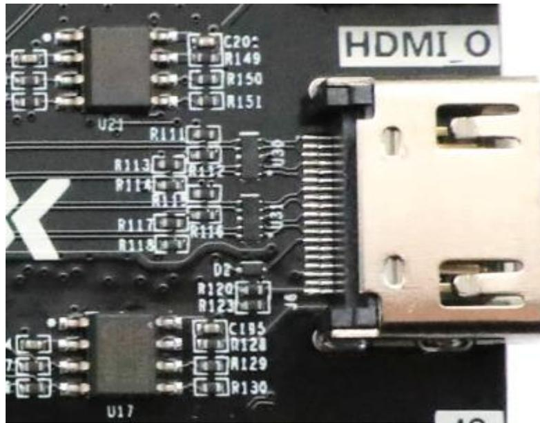
Figure 9-5: HDMI Input Interface on the FPGA Board
