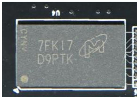
Figure 6-2: The DDR3 on the FPGA Board
