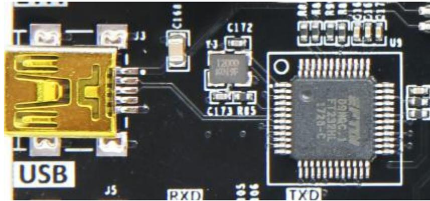
Figure 11-2: USB 2.0 part on the FPGA Board
