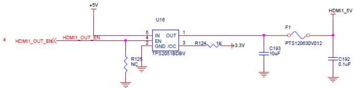
Figure 9-2: HDMI +5V Output Schematic
