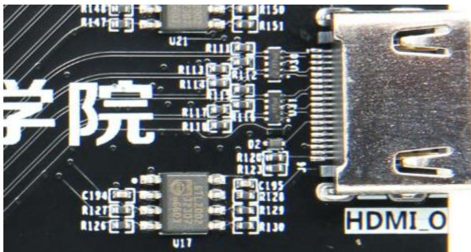
Figure 9-4: HDMI Output Interface on the FPGA Board
