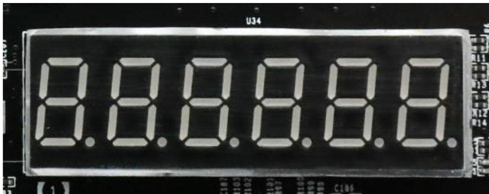
Figure 15-3: Digital Tube on the FPGA Board
