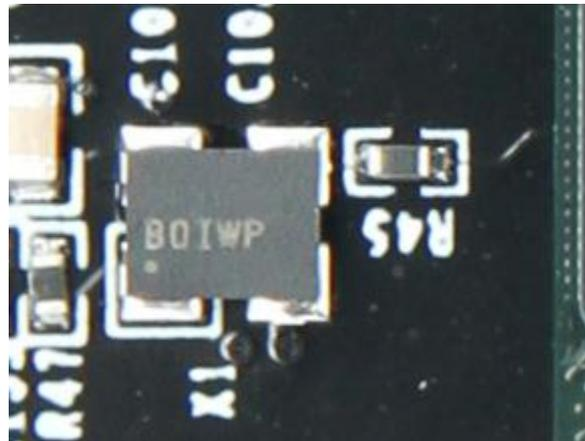
Figure 5-2: 50M active crystal oscillator on the FPGA Board
