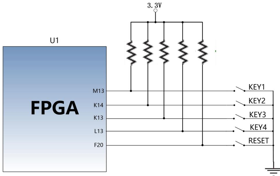
Figure 20-1: Key Schematic
