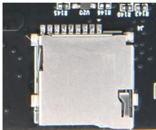
Figure 12-2: SD Card Slot on the FPGA Board
