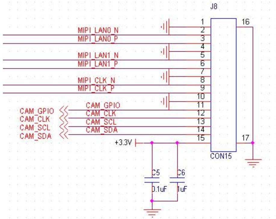
Figure18-1: FPC Expansion Ports Schematic
