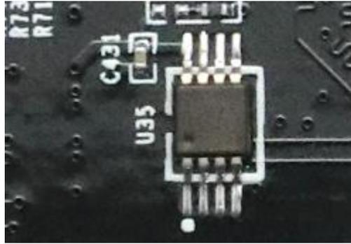
Figure 16-2: LM75 Sensor on the FPGA Board
