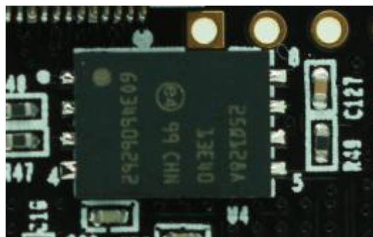
Figure 7-2: QSPI on the FPGA Board
