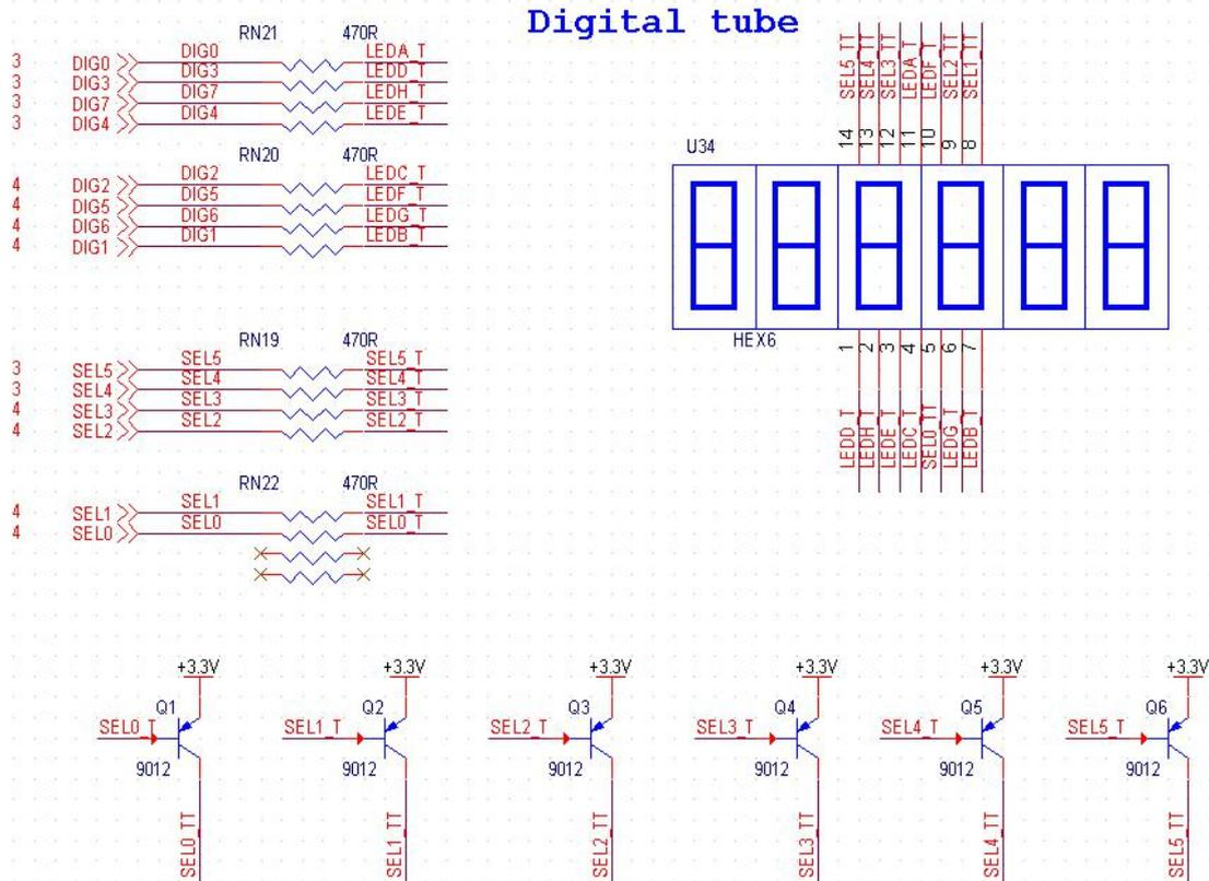
Figure 15-2: Digital Tube Schematic
