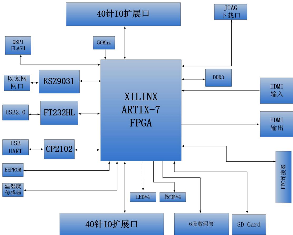
Figure 1-1: The Schematic Diagram of the AX7035
