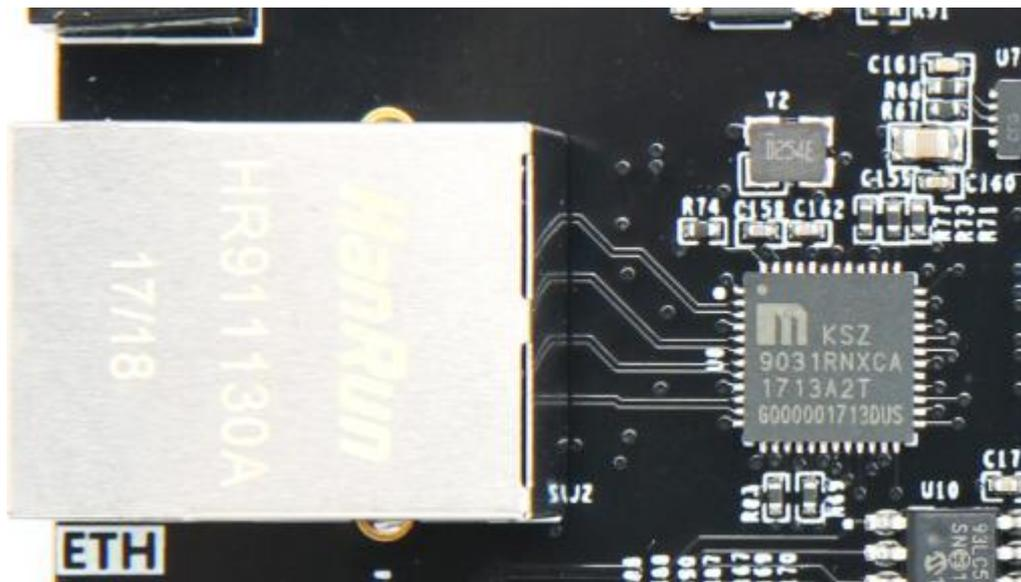
Figure 8-2: Gigabit Ethernet interface on the board
