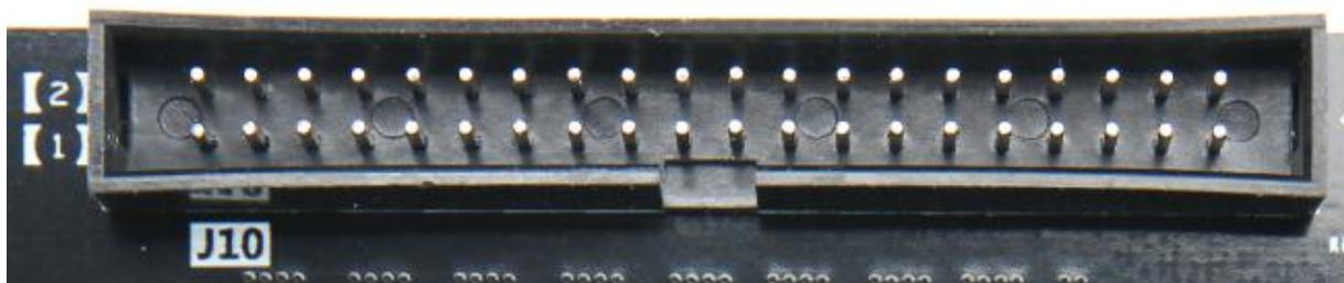
Figure 17-4: Expansion header J10 on the FPGA Board
