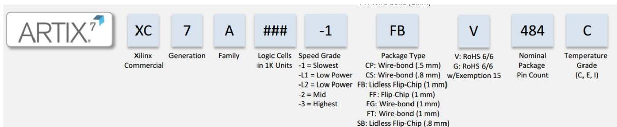
Figure 4-1: The Specific Chip Model Definition of ARTIX-7 Series
