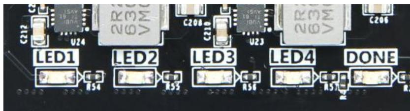
Figure 21-2: The User LEDs on the FPGA Board
