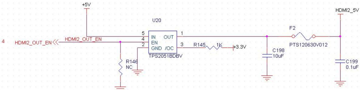
Figure 10-2: HDMI2 power control circuit
