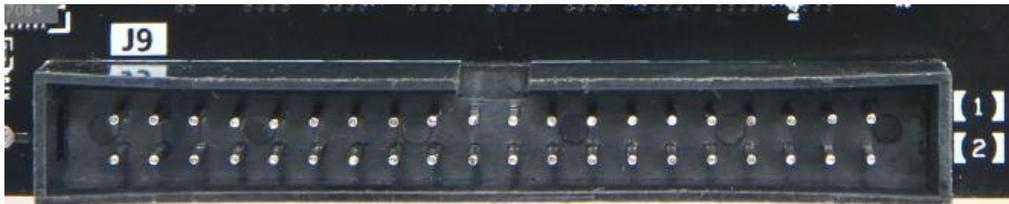
Figure 17-2: Expansion header J9 on the FPGA Board
