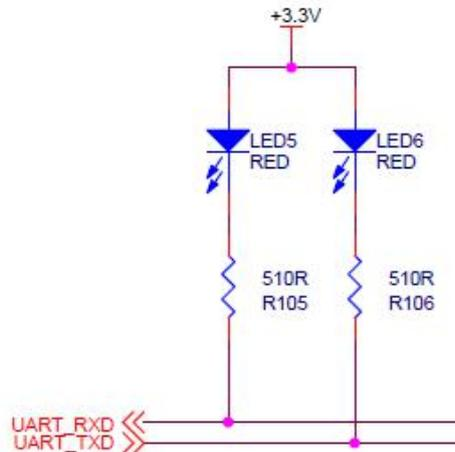
Figure 13-3: Serial Port communication LED Indicators Schematic
