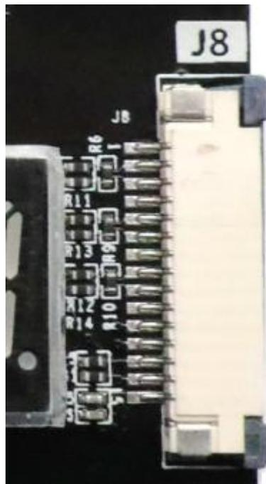
Figure18-2: FPC Expansion Ports on the FPGA Board
