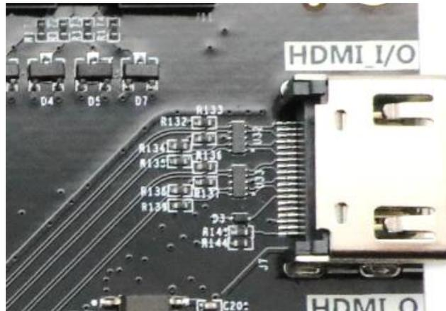
Figure 10-4: HDMI Input Interface on the board
