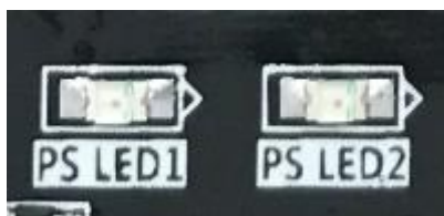
Figure 6-15: PS User LEDs on the FPGA Board
