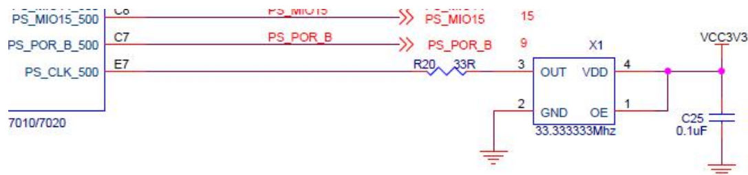
Figure 5-1: Active crystal oscillator to the PS section
