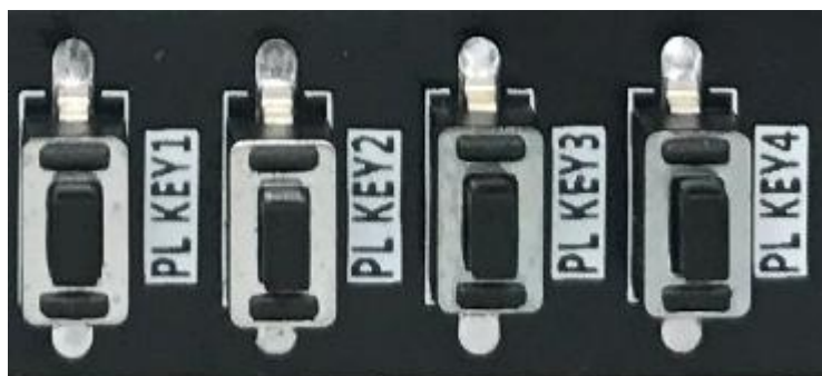
Figure 7-16: PL User Buttons on the FPGA Board
