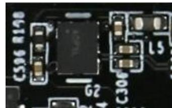
Figure 2-6-5: Programmable Clock Source on the AX7Z100 FPGA Core Board
