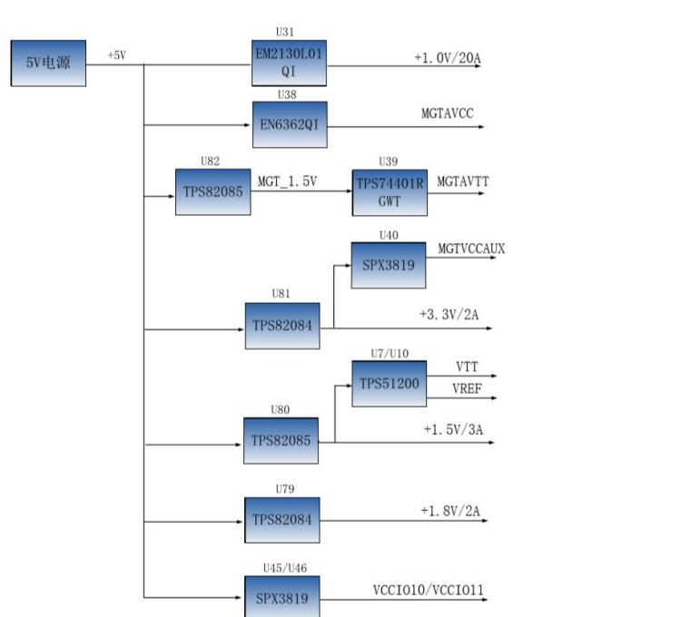
Figure 2-9-1: Power interface section in the schematic
