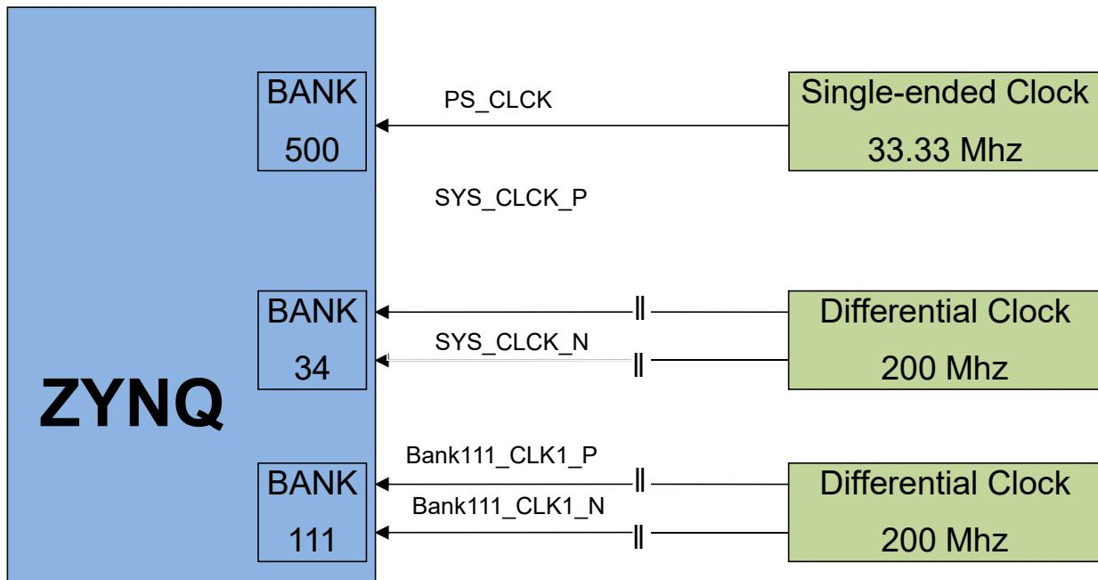
Figure 2-6-1: Clock source in the Core Board
