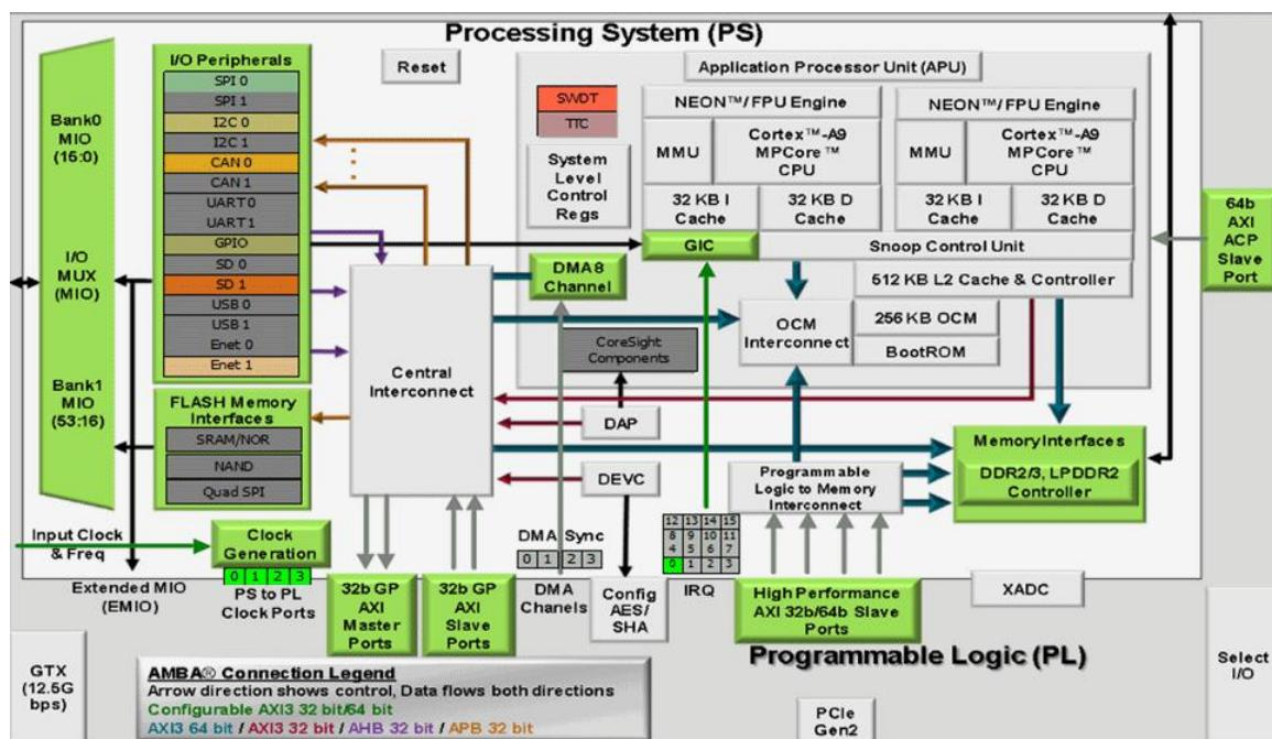
Figure 2-2-1: Overall Block Diagram of the ZYNQ7000 Chip
