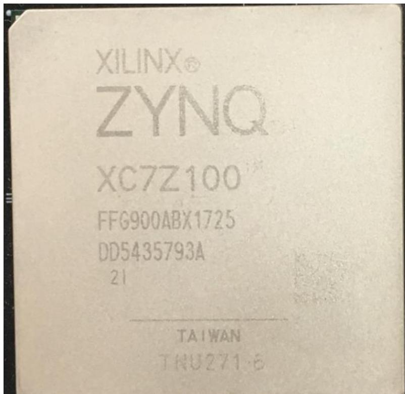
Figure 2-2-3: The XC7Z100 chip used on the Core Board
