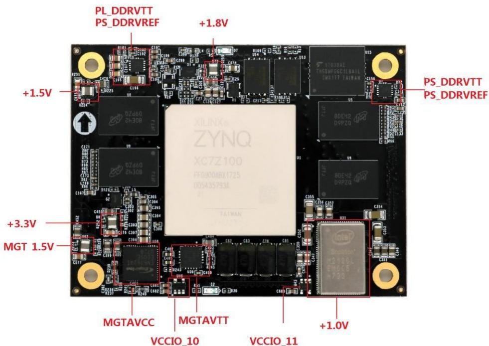
Figure 2-9-2: Power Supply on the AX7Z100 Core Board
