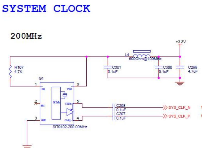
Figure 2-6-3: PL system clock source
