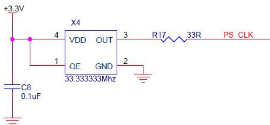
Figure 2-6-2: Active crystal oscillator to the PS section
