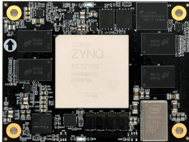
Figure 2-1-1: AC7Z100 Core Board (Front View)
