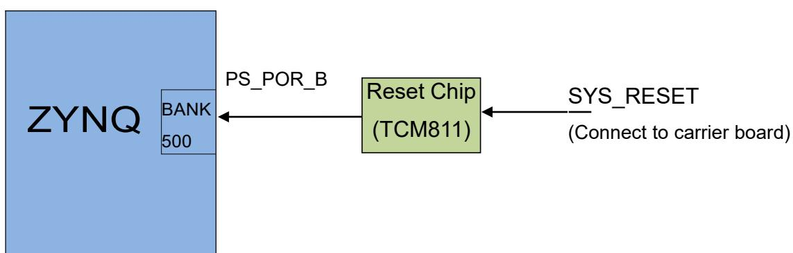
Figure 2-8-1: Reset circuit connection diagram
