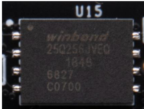
Figure 2-4-2 is the QSPI Flash on the core board
