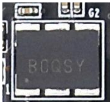
Figure 3-4: 125MHz Active Differential Crystal on the Core Board
