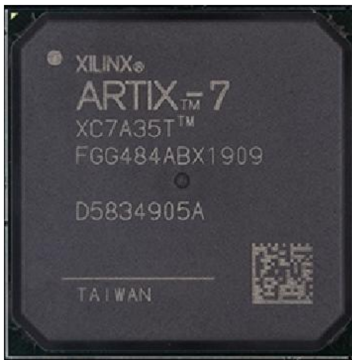
Figure 2-2: FPGA chip on board
